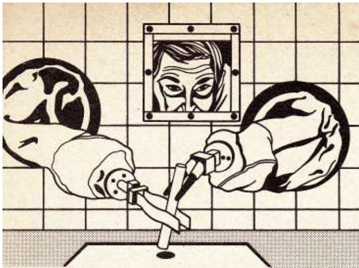
Remote handling of radio-active materials. Most radio-active materials are too dangerous to handle directly. Surprisingly perhaps, uranium and plutonium can be touched with bare hands, but only in their metallic 'non-dust' form.
